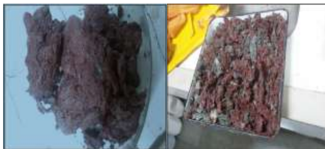
FIG.1 APPEARANCE OF PAINT-SLUDGE
